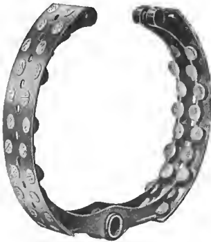
Fig. 3—Shoe of expanding band clutch, fitted with cork inserts.
